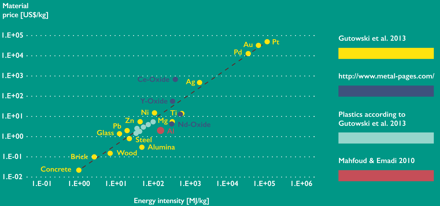
Fig. 5 | Material price as a function of energy intensity
